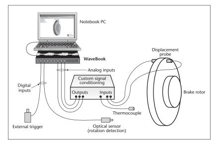
The system block diagram for dynamic brake testing of warranty returned parts is relatively simple and perhaps belies the importance and significance of the test. However, the IOtech WaveBook measurement system equipped with Digital Metrology's custom analysis software can detect displacements in microns and sort out the very few truly defective parts from the greater number of misdiagnosed parts.
